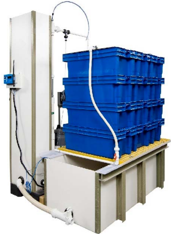
Figure 1: Holding unit with stacked totes for short term holding. Unit dimensions with insulation panels: 230 x 170 cm H: 247 cm
